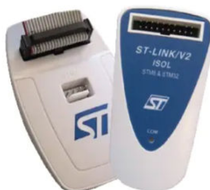
Figure 1. ST-LINK/V2 tool for microcontroller programming
