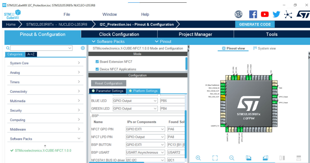
Figure 15. STM32CubeMX Pinout & Configuration tab and Additional pack settings for NFC07A1_I2CProtection example
