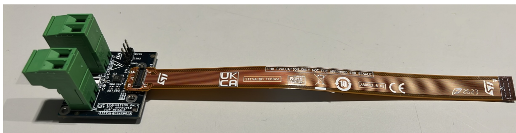
Figure 2. Expansion board and flex cable
