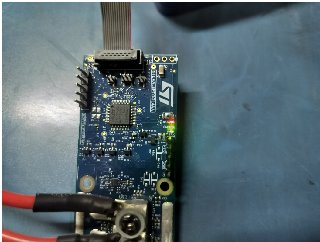
Figure 19. Both LEDs on during basic checks before running the motor
