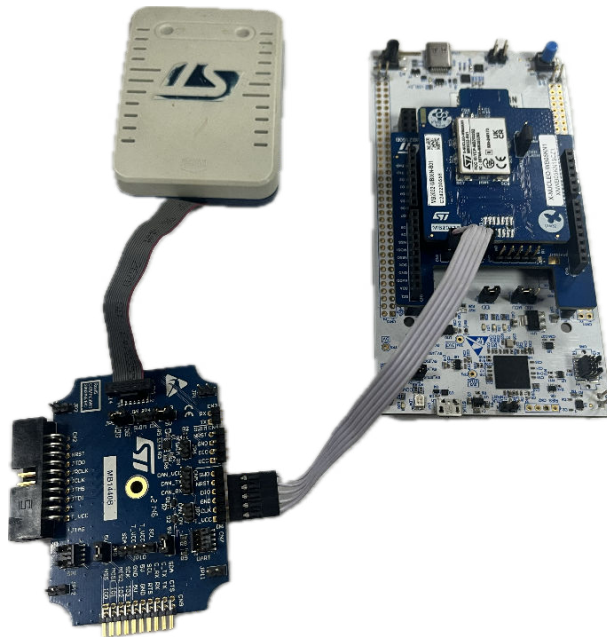
Figure 6. X-NUCLEO-WB05KN1 connected to ST-LINK/V3
