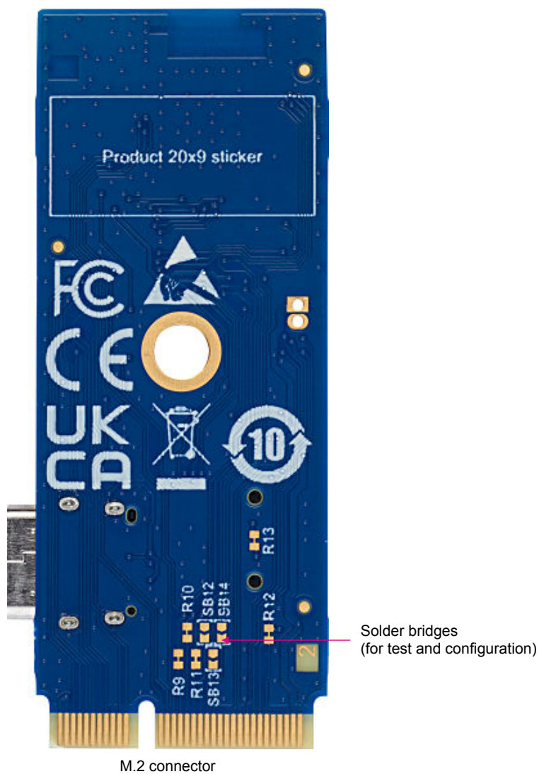
Figure 5. B-WBA5M-WPAN PCB layout bottom side
