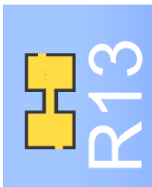
Figure 13. Footprint of a short-circuited resistor
