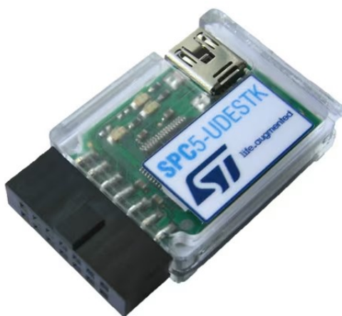
Figure 4. SPC5-UDESTK USB/JTAG interface
