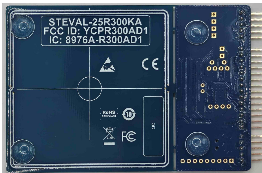
Figure 8. STEVAL-25R300KA expansion board layout (bottom view)
