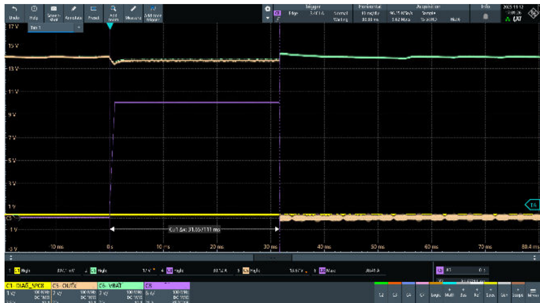
Figure 42. OUT2, VNF9D1M5Q STi 2 Fuse regular functionality test ( I_{\text{nom}} = 21 \text{ A} , t_{\text{nom}} = 1 \text{ s} ) (2 of 3)
