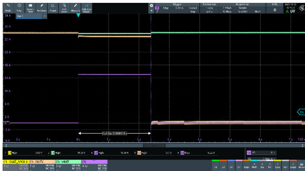
Figure 64. OUT9 (@15 A load current), VNF9Q20SF STi 2 Fuse regular functionality test ( I_{nom} = 6\text{ A} , t_{nom} = 300\text{ s} ) (3 of 3)
