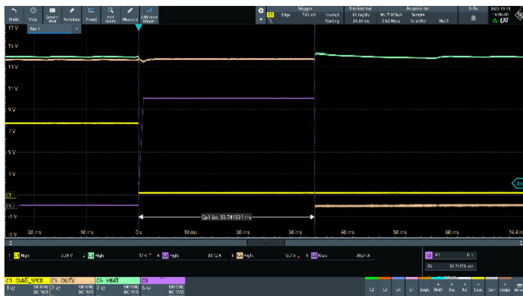
Figure 36. OUT0, VNF9D1M5Q STi 2 Fuse regular functionality test ( I_{nom} = 21\text{ A} , t_{nom} = 1\text{ s} ) (2 of 3)
