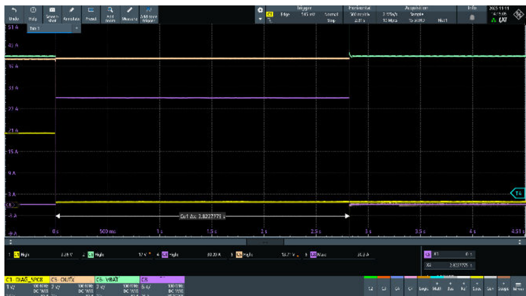
Figure 40. OUT1, VNF9D1M5Q STi 2 Fuse regular functionality test ( I_{nom} = 16\text{ A} , t_{nom} = 172\text{ s} ) (3 of 3)
