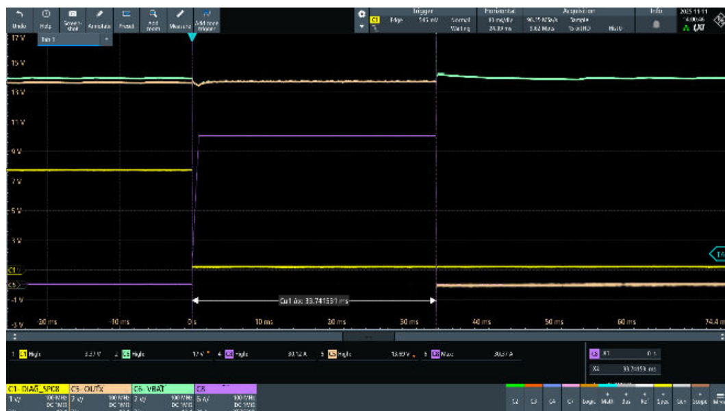
Figure 35. OUT0, VNF9D1M5Q STi 2 Fuse regular functionality test ( I_{nom} = 21\text{ A} , t_{nom} = 1\text{ s} ) (1 of 3)
