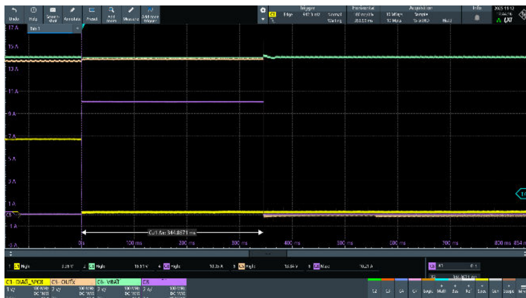
Figure 47. OUT4, VNF9D5SF STi 2 Fuse regular functionality test ( I_{nom} = 4\text{ A} , t_{nom} = 44\text{ s} ) (1 of 3)
