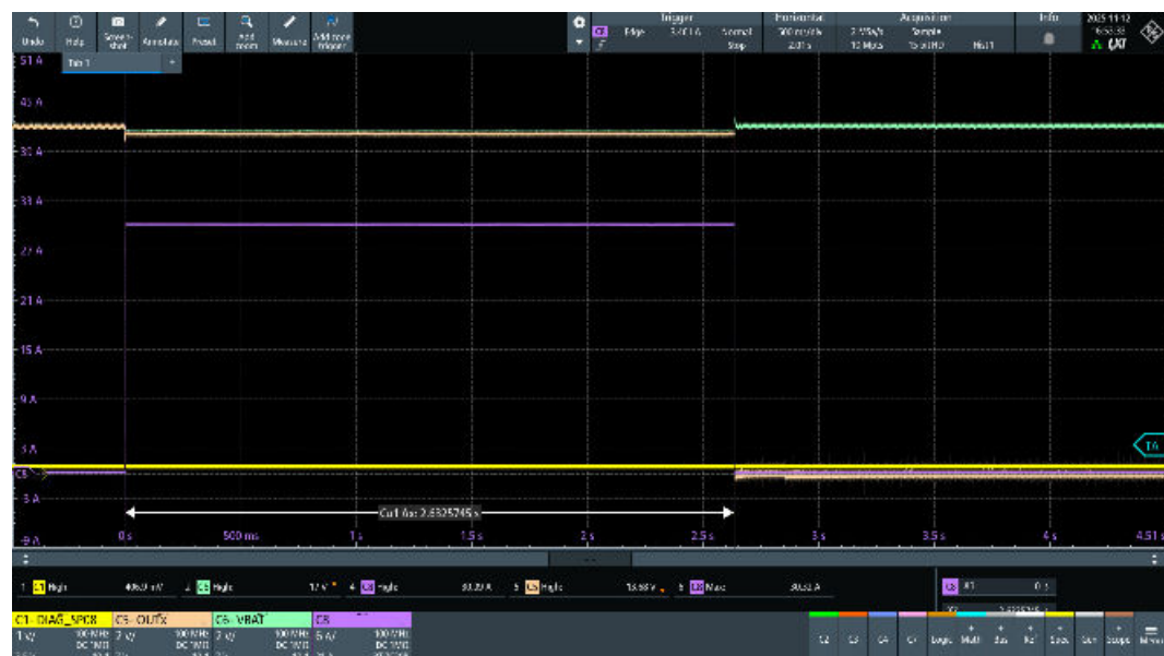
Figure 46. OUT3, VNF9D1M5Q STi 2 Fuse regular functionality test ( I_{nom} = 16\text{ A} , t_{nom} = 172\text{ s} ) (3 of 3)
