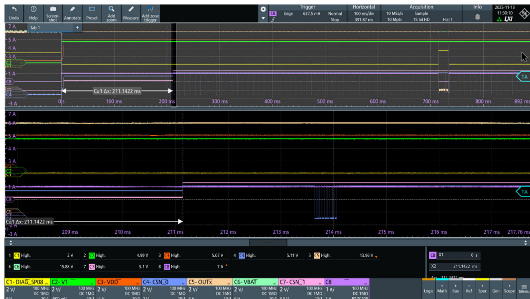
Figure 27. OUT0 wake-up, CSN0 and CSN1 reach 5 V and CSN0 start communication
