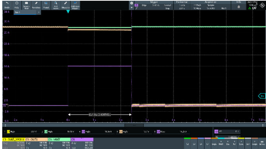
Figure 60. OUT8, VNF9Q20SF STi 2 Fuse regular functionality test ( I_{\text{nom}} = 6 A, t_{\text{nom}} = 300 s) (2 of 3)
