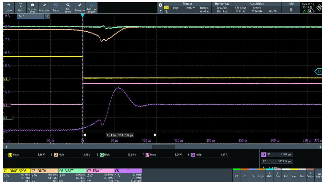
Figure 119. OUT6, P-channel companion chip activating VNF9Q20SF device
