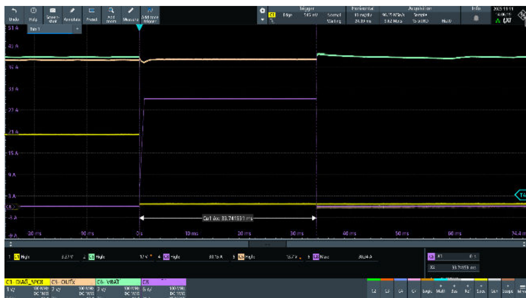
Figure 37. OUT0, VNF9D1M5Q STi 2 Fuse regular functionality test ( I_{nom} = 21\text{ A} , t_{nom} = 1\text{ s} ) (3 of 3)
