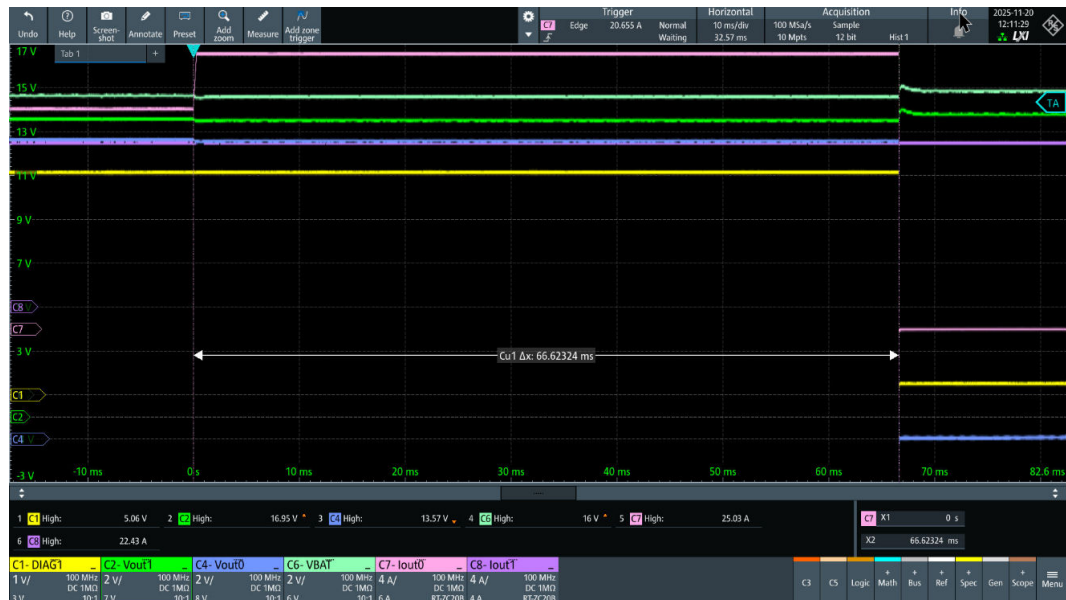
Figure 104. VNF9D1M5Q (dev0), OUT0 and OUT1 independent channel operation
