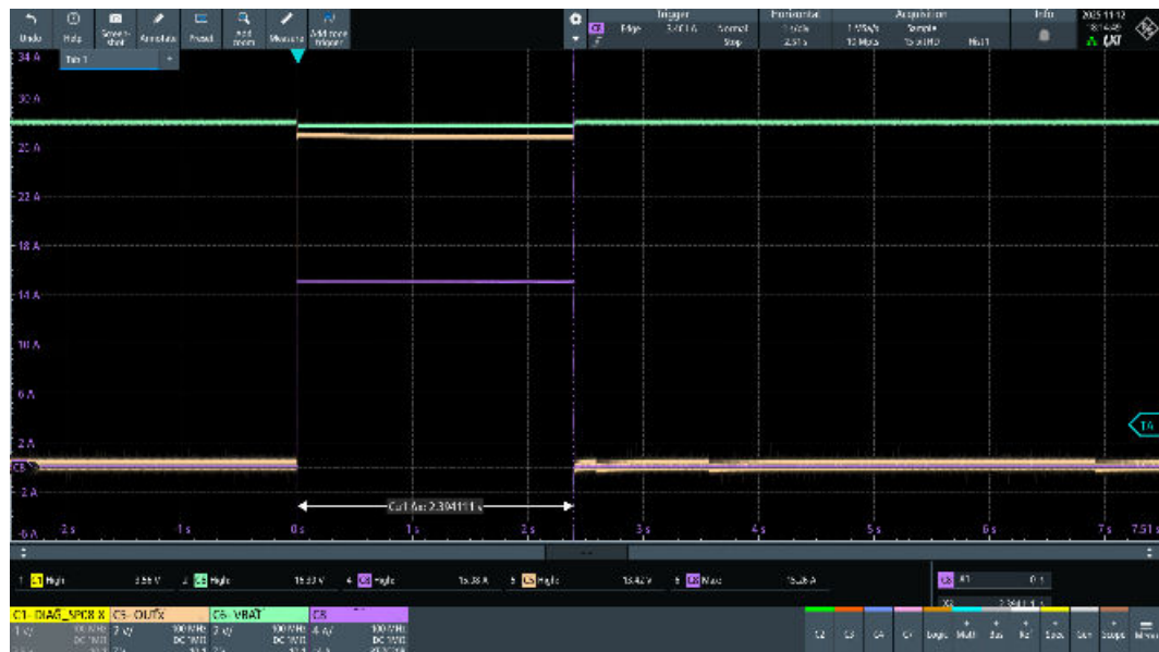
Figure 63. OUT9 (@15 A load current), VNF9Q20SF STi 2 Fuse regular functionality test ( I_{nom} = 6\text{ A} , t_{nom} = 300\text{ s} ) (2 of 3)
