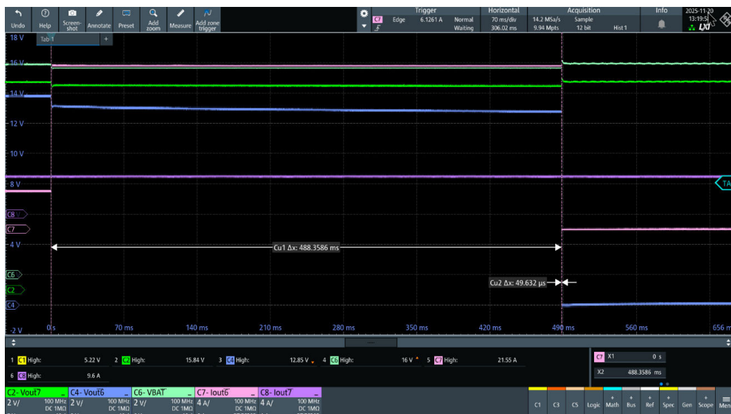
Figure 111. VNF9Q20SF, OUT6 and OUT7 independent channel operation (details of latch off time)
