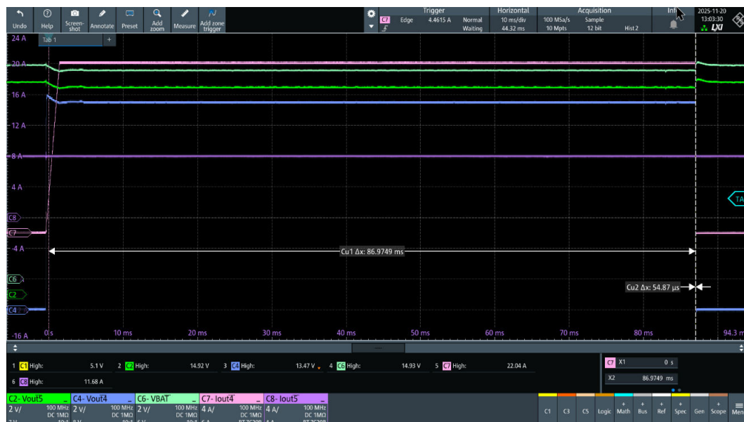
Figure 109. VNF9D5SF, OUT4 and OUT5 independent channel operation (details of latch off time)
