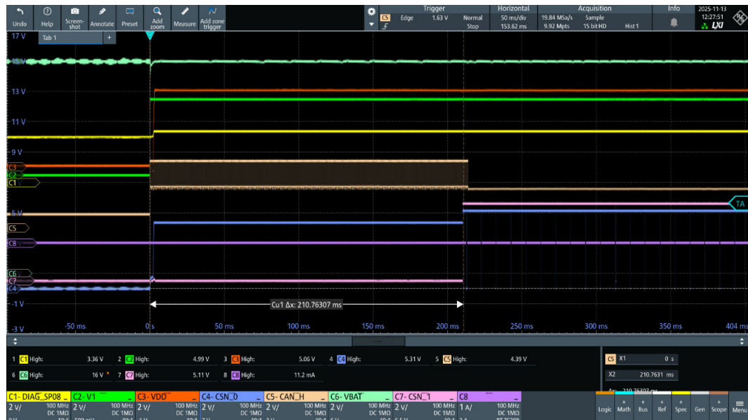
Figure 32. Module wake-up through CAN ( t_{CSN0-1(5V)} = 210.73 \text{ ms} )
