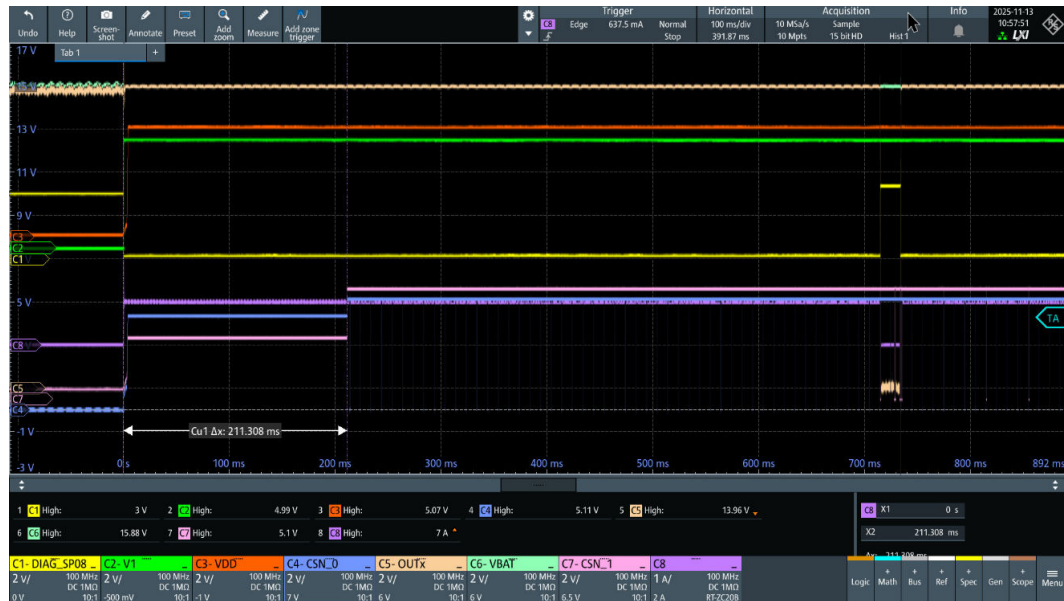
Figure 26. OUT0 wake-up, DIAG_SP08 signal low and CSN0 and CSN1 reach 5 V ( t_{CSN0-1(5\text{ V})} = 211.3\text{ ms} )
