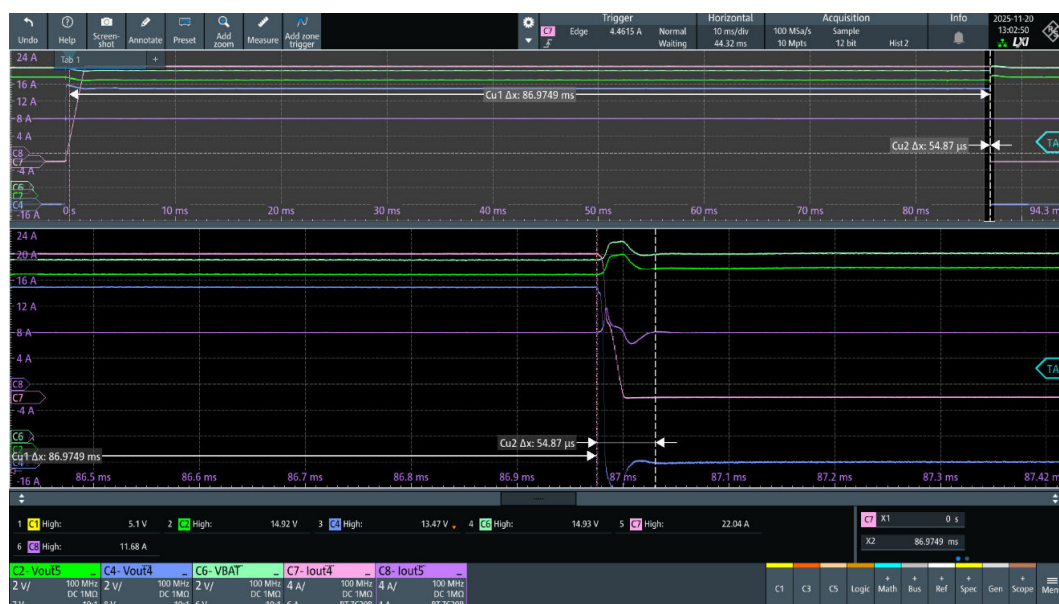
Figure 109. VNF9D5SF, OUT4 and OUT5 independent channel operation (details of latch off time)
