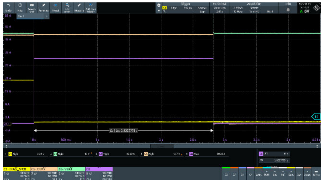
Figure 40. OUT1, VNF9D1M5Q STi 2 Fuse regular functionality test ( I_{nom} = 16\text{ A} , t_{nom} = 172\text{ s} ) (3 of 3)
