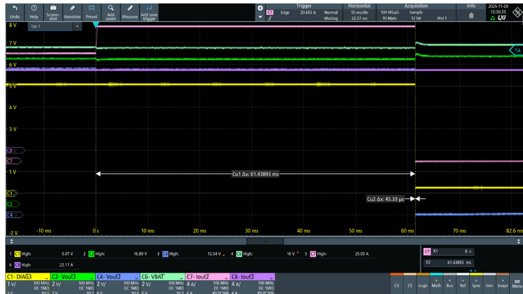
Figure 107. VNF9D1M5Q (dev1), OUT2 and OUT3 independent channel operation (details of latch off time)
