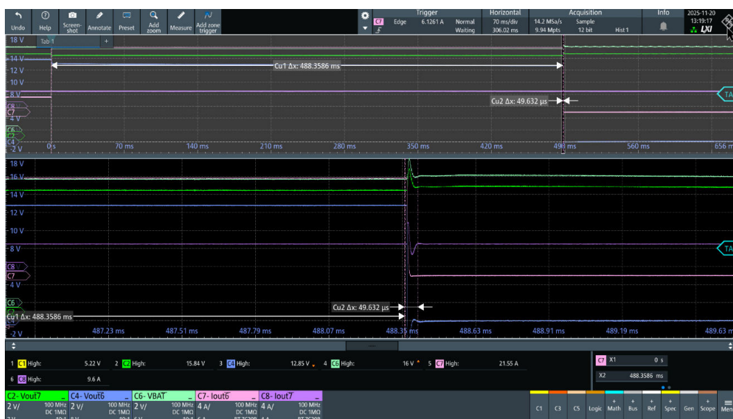
Figure 111. VNF9Q20SF, OUT6 and OUT7 independent channel operation (details of latch off time)
