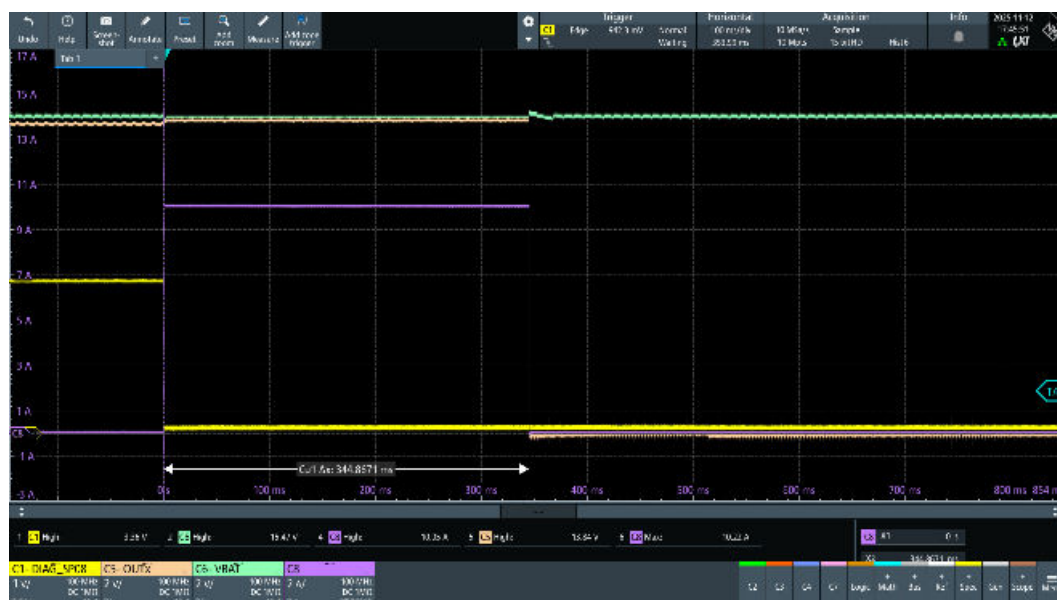
Figure 48. OUT4, VNF9D5SF STi 2 Fuse regular functionality test ( I_{nom} = 4\text{ A} , t_{nom} = 44\text{ s} ) (2 of 3)
