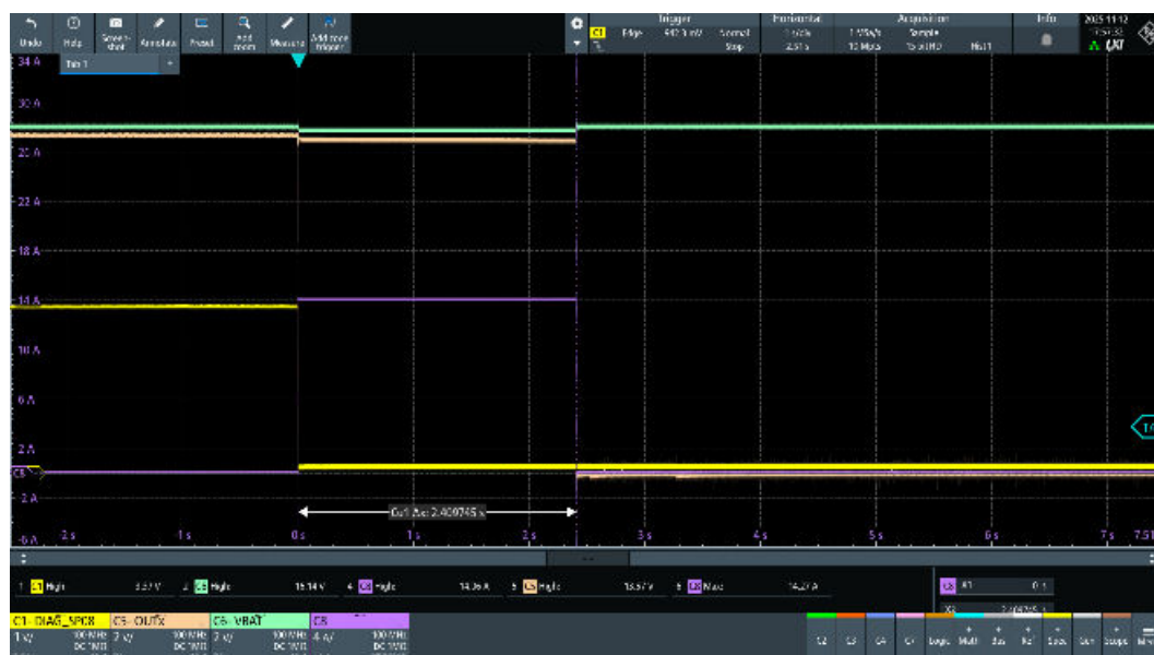
Figure 54. OUT6, VNF9Q20SF STi 2 Fuse regular functionality test ( I_{nom} = 6\text{ A} , t_{nom} = 300\text{ s} ) (2 of 3)
