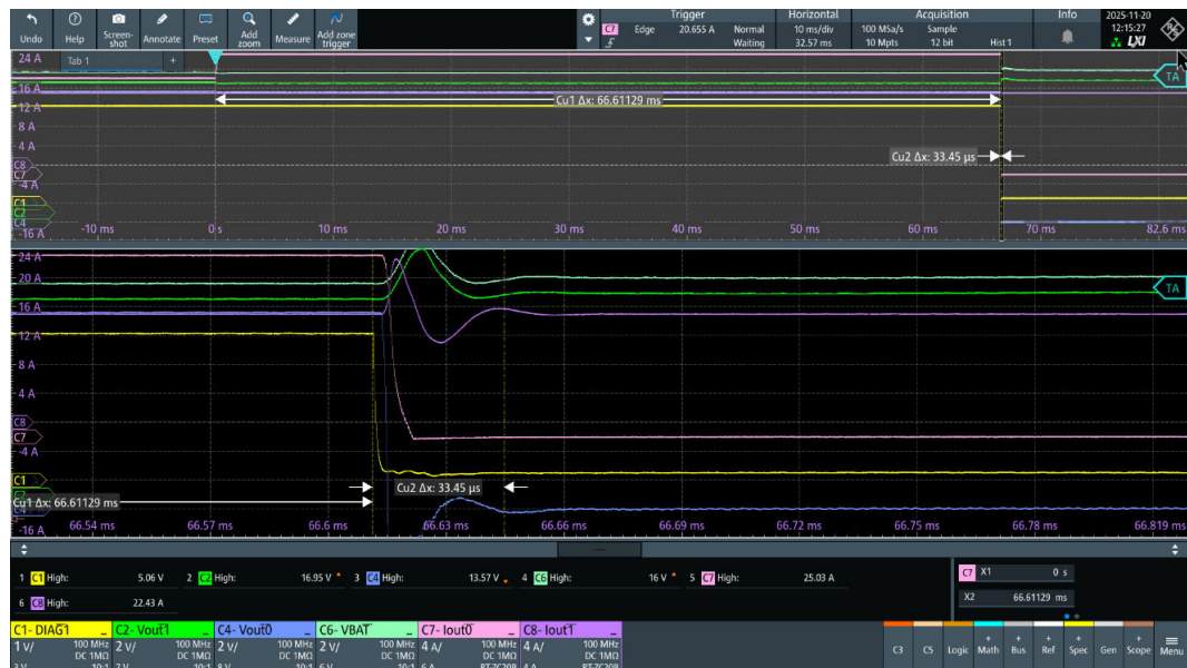
Figure 105. VNF9D1M5Q (dev0), OUT0 and OUT1 independent channel operation (details of latch off time)
