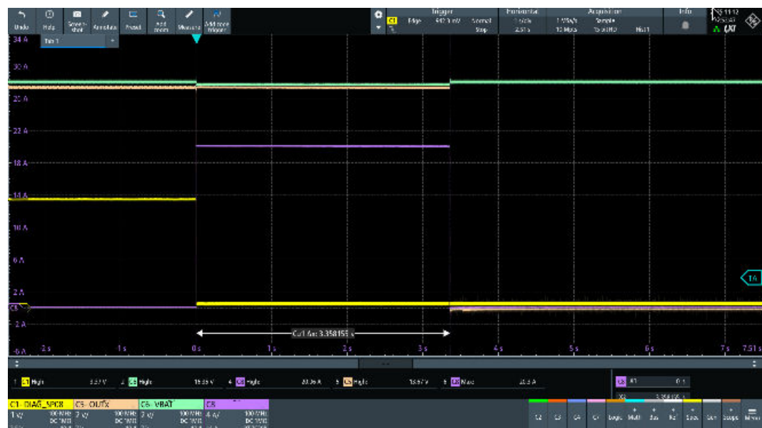
Figure 52. OUT5, VNF9D5SF STi 2 Fuse regular functionality test ( I_{nom} = 10\text{ A} , t_{nom} = 214\text{ s} ) (3 of 3)
