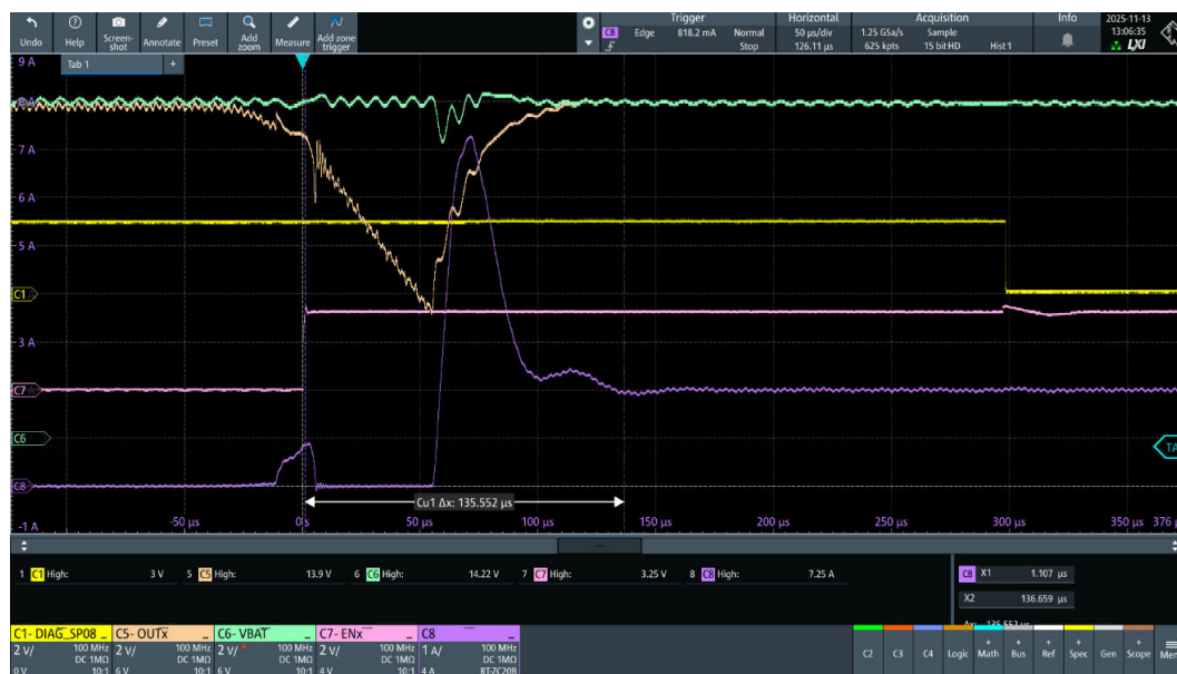
Figure 116. OUT3, P-channel companion chip activating VNF9D1M5Q device
