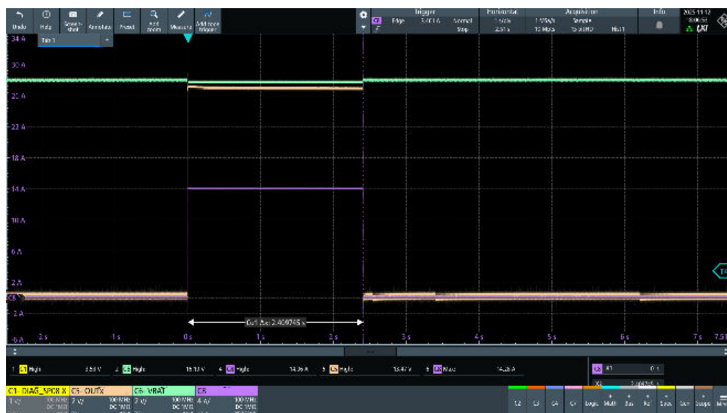
Figure 61. OUT8, VNF9Q20SF STI 2 Fuse regular functionality test ( I_{nom} = 6\text{ A} , t_{nom} = 300\text{ s} ) (3 of 3)
