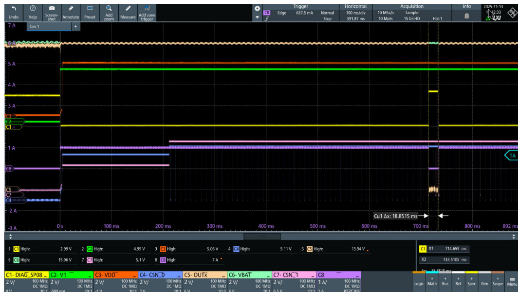
Figure 29. OUT2 wake-up - DIAG_SP08, CSN0, CSN1, and output signals
