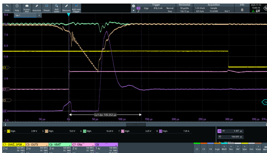
Figure 115. OUT2, P-channel companion chip activating VNF9D1M5Q device
