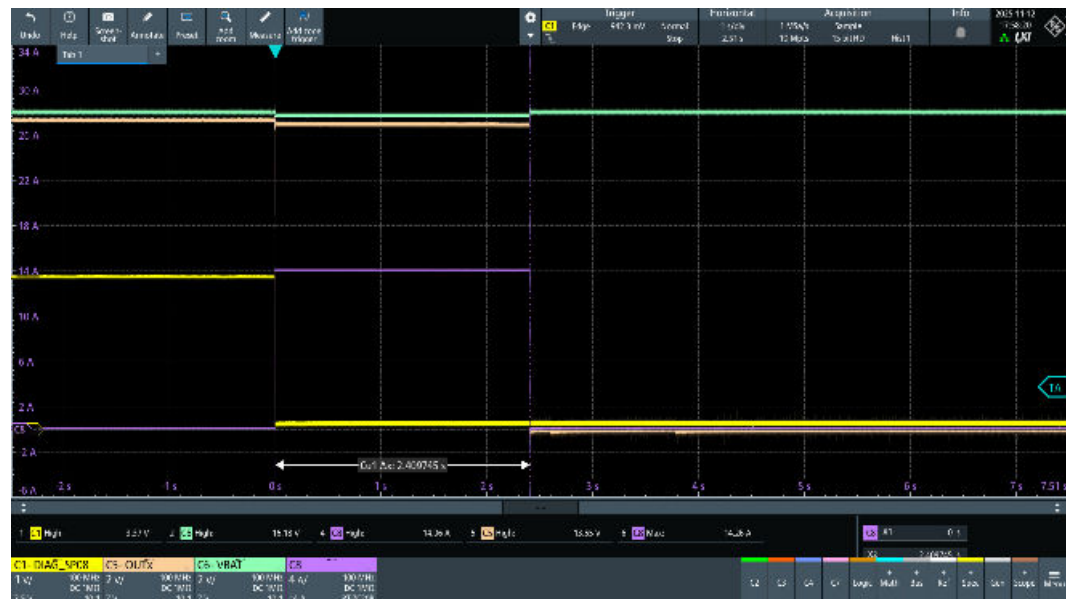
Figure 55. OUT6, VNF9Q20SF STi 2 Fuse regular functionality test ( I_{nom} = 6\text{ A} , t_{nom} = 300\text{ s} ) (3 of 3)
