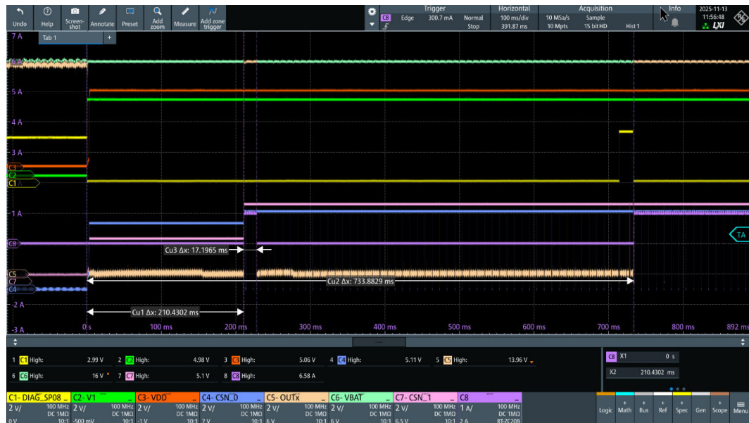
Figure 30. OUT4 wake-up (tCSN0-1(5 V) = 210.43 ms)
