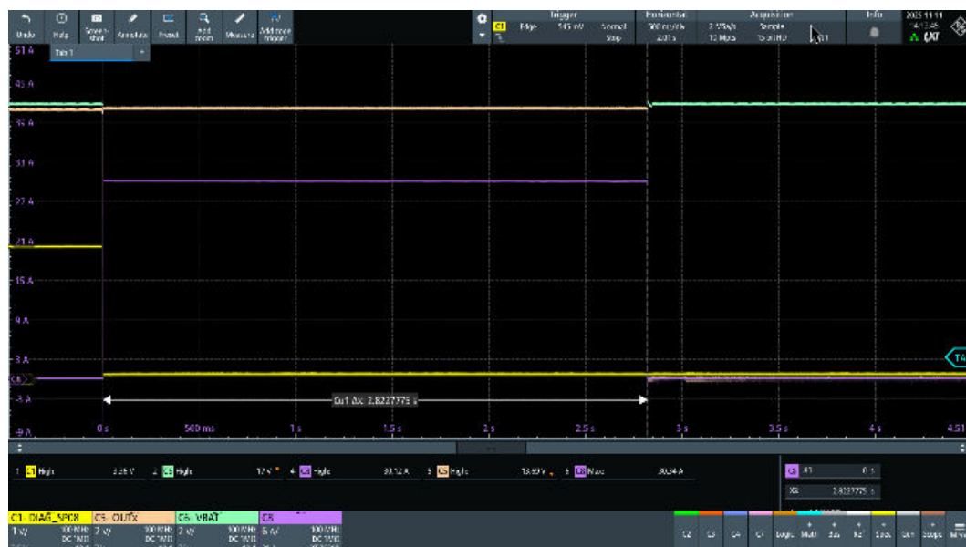
Figure 38. OUT1, VNF9D1M5Q STi 2 Fuse regular functionality test ( I_{nom} = 16\text{ A} , t_{nom} = 172\text{ s} ) (1 of 3)
