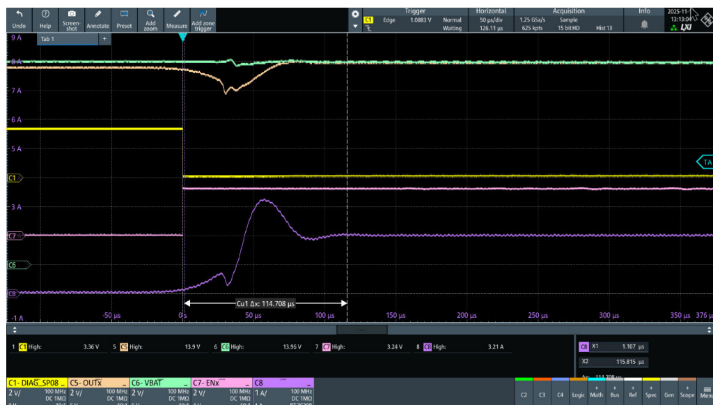
Figure 120. OUT7, P-channel companion chip activating VNF9Q20SF device
