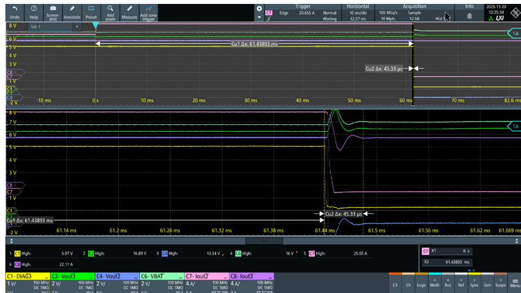
Figure 107. VNF9D1M5Q (dev1), OUT2 and OUT3 independent channel operation (details of latch off time)
