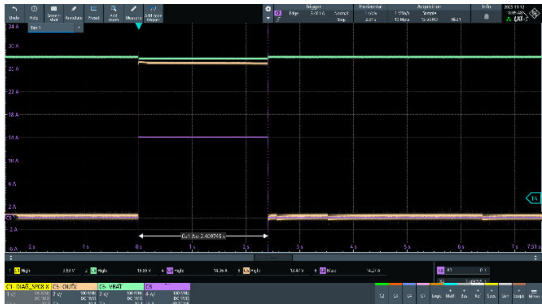
Figure 60. OUT8, VNF9Q20SF STi 2 Fuse regular functionality test ( I_{\text{nom}} = 6 A, t_{\text{nom}} = 300 s) (2 of 3)
