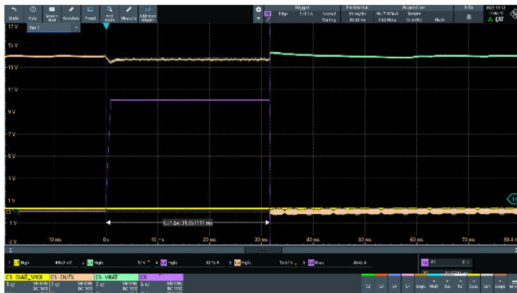
Figure 43. OUT2, VNF9D1M5Q STi 2 Fuse regular functionality test ( I_{nom} = 21\text{ A} , t_{nom} = 1\text{ s} ) (3 of 3)
