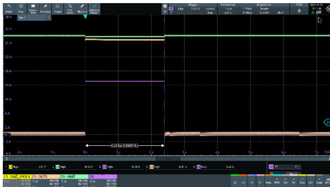
Figure 62. OUT9 (@15 A load current), VNF9Q20SF STI 2 Fuse regular functionality test ( I_{nom} = 6\text{ A} , t_{nom} = 300\text{ s} ) (1 of 3)
