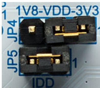
Figure 7. STM32 Nucleo VDD configuration (JP4)
