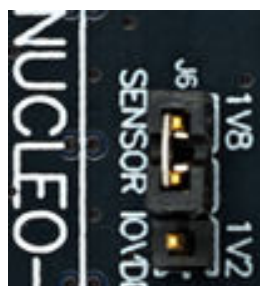
Figure 9. SENSOR IOVDD jumper configuration (J6 to 1V8)
