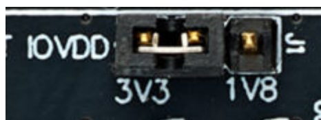
Figure 8. EXT IOVDD jumper configuration (J1)
