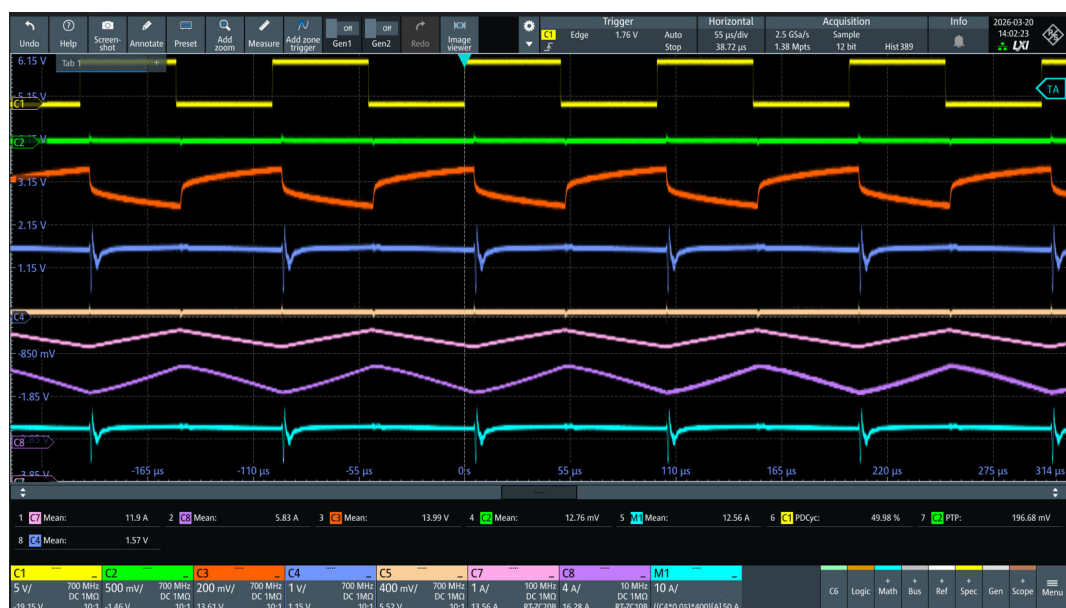
Figure 33. AEK-MOT-8DCMH98 oscilloscope capture of CH1 and CH2 full bridge at 50% PWM
