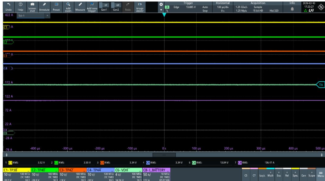
Figure 42. AEK-MOT-8DCMH98 oscilloscope capture of the 4 full bridges at 100% PWM
