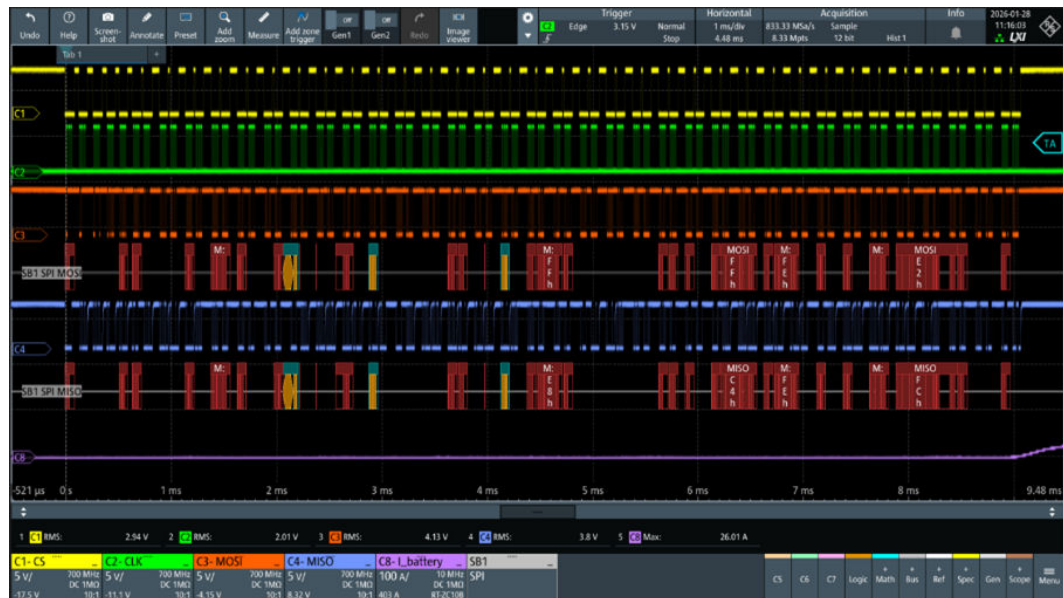
Figure 25. SPI signals for L99MH94
