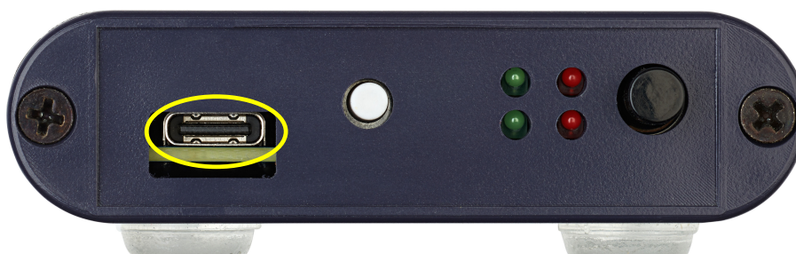
Figure 6. USB Type-C® position
