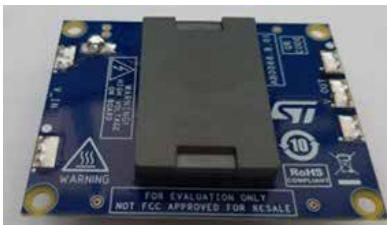
Figure 21. Planar transformer for LLC
