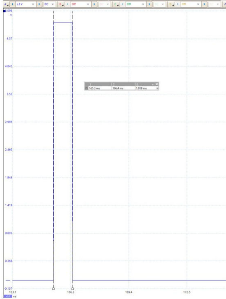
Figure 12. Enable pulse signal waveform generated by an external MCU connected to the AEK-POW-LDOV02J
