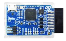
A compact, cost-effective USB-to-JTAG debugger/ programmer dongle that ensures short development times through easy-to-use hardware and software fully integrated into SPC5-Studio and AutoDevKit Studio IDEs.
