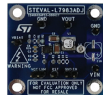
STEVAL-L7983ADJ 12 V/0.3 A降压DC/DC转换器 (VIN = 12 - 60 V)
