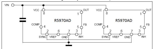
Figure 20. Synchronization example
