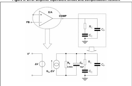
The poles of this transfer function are (if  $C_c >> C_0 + C_P$ ):
