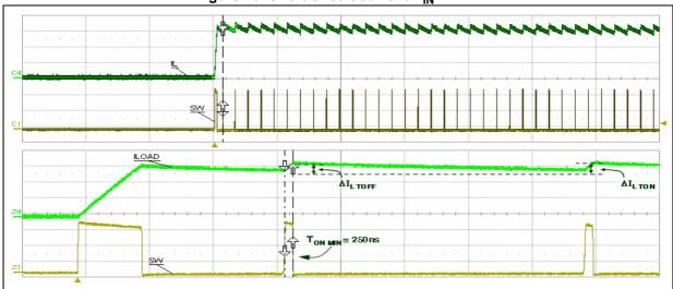
Figure 17. Short-circuit current  $V_{IN}$  = 36 V
