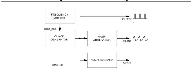
Figure 4. Oscillator circuit block diagram
