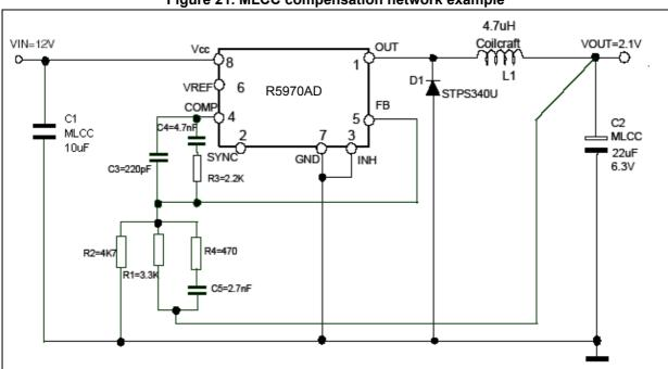
Figure 21. MLCC compensation network example
