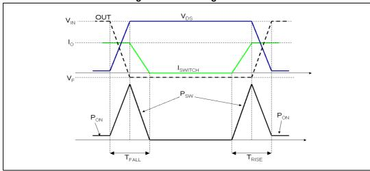
Figure 14. Switching losses
