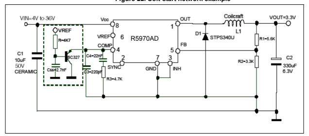
Figure 22. Soft-start network example
