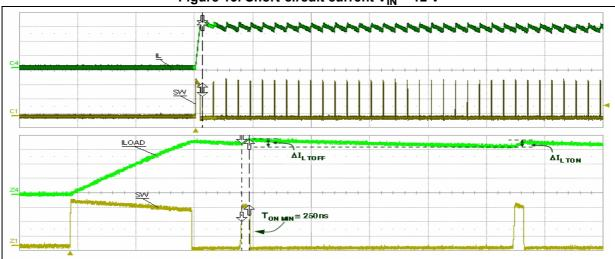
Figure 15. Short-circuit current  $V_{IN} = 12 \text{ V}$
